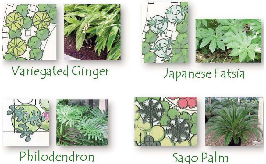
Figure 30. Plan symbols may be modified to reflect texture or other plant characteristics. This allows the species to be quickly recognizable when you are reviewing your planting plan. Image and planting symbols by Pat Drackett.
